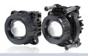
LED low beam headlamp Module 60 LED
